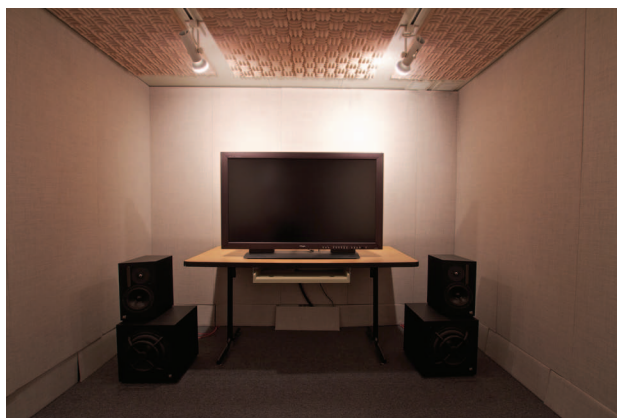
[FIG8] A picture of the viewing environment should be included in the final report. This sample environment shows a sound isolation booth. A Blu-ray player outside the room plays audiovisual sequences on a broadcast-quality monitor and speakers.
